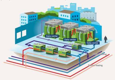
At normal operation, the heat pumps use the district cooling network's return line and cools it down to the desired temperature for use in the data centre. The heat produced is delivered to the district heating supply line, thus making the district heating network the heat sink for the heat pump. The total cooling capacity is approximately 1,200 kW when district cooling at 5.5 °C and district heating at 68 °C is delivered. The heating effect corresponds to approximately 1,600 kW.
