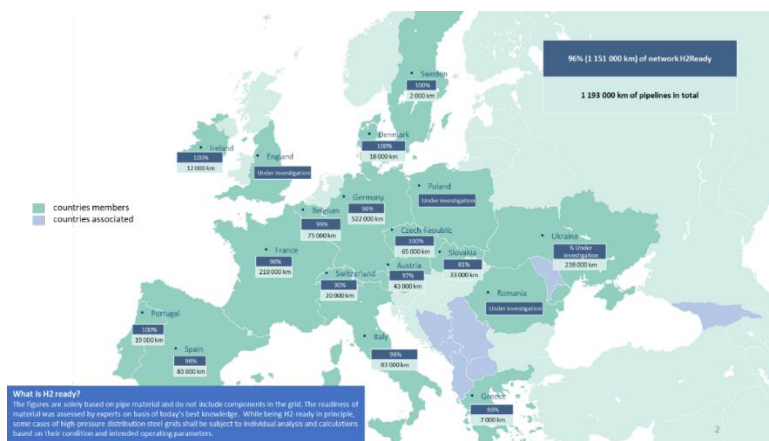
Figure 30: Readiness for pipeline's repurposing potential. Source: Ready4H2 146 .
