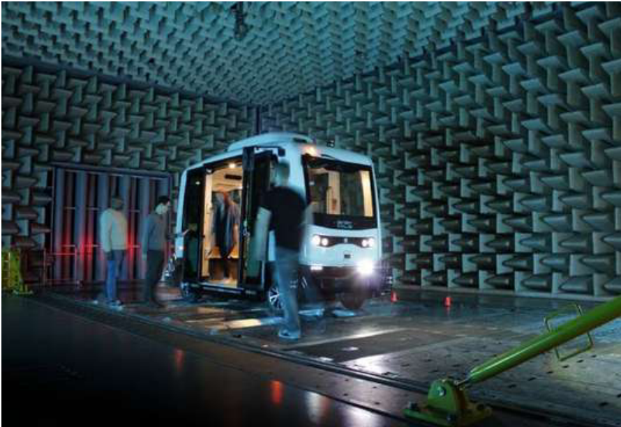
Autonomous shuttle in KIT's acoustic four-wheel roller dynamometer
