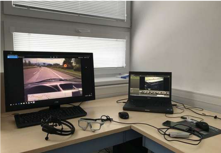
Eyetracking glasses for capturing driver's glance to monitor driver's behaviour; they are used together with an electroencephalograph device, which measures brain activity of a driver.
