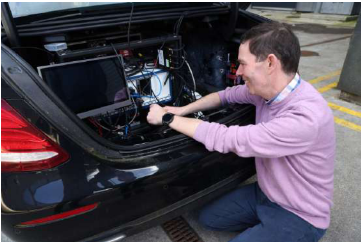
Optimising camera, radar, and lidar inputs in a semi-autonomous test vehicle as part of Lero's Blended Autonomous Vehicle project'
