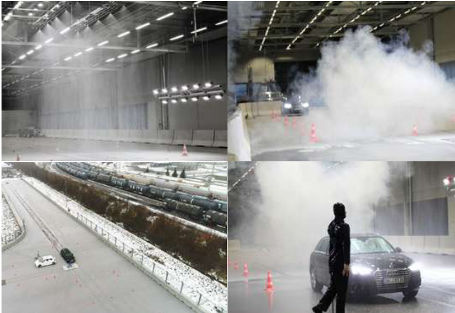
Outdoor and Indoor CARISSMA Test Facilities under weather conditions ( Rain and Fog Simulation Tests )
